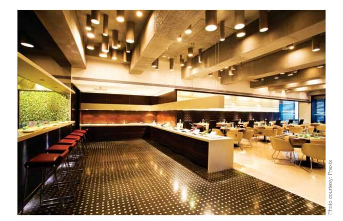
Terrazzo tiles are possible to make with creative inserts ranging from stone to mirrors. Featured on this page are tiles using mirrors as inserts.
